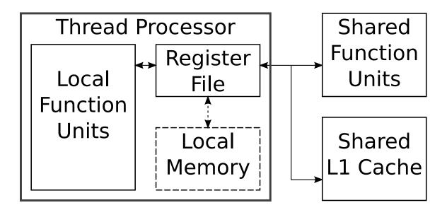
Figure 2.2: Thread Processor Block Diagram
