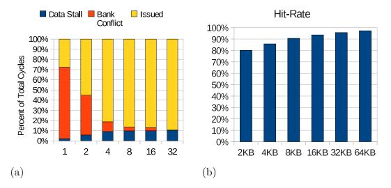
**Figure 5.5**: L1 Data Cache Performance for a Single TM with Over-Provisioned Functional Units and Instruction Cache. (a) Issue Rate for Varying Banks in a 2KB Data Cache. (b) Deache Hit%, 8-banks and Varying Capacities.
