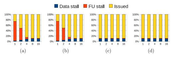
**Figure 5.6**: Effect of Shared Functional Units on Issue Rate Shown as a Percentage of Total Cycles. (a) FP Add/Sub (13% of Issued Insts). (b) FP Multiply (13% of Issued Insts). (c) FP Inverse Square Root (0.4% of Issued Insts). (d) Int Multiply (0.3% of Issued Insts)
