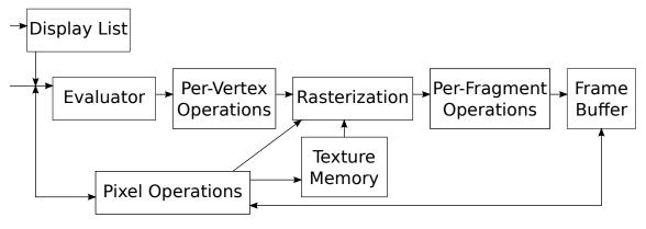
Figure 1.2: OpenGL Pipeline
