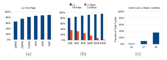
Figure 5.7: L2 Performance for 16 Banks and TMs with the Top Configuration Reported in Table 5.9. (a) Hit-rate for Varying L2 Capacities with 20 TMs Connected to Each L2. (b) Percentage of Cycles not Issued Due to L2 Bank Conflicts for Varying L1 Capacities (and Thus Hitrates) for 20 TMs. (c) L2 Bank Conflicts for a Varying Number of TMs Connected to Each L2. Each TM Has a 64KB L1 Cache with 95% Hitrate.
