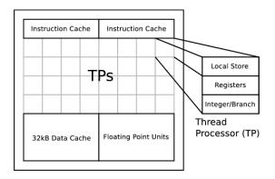
Figure 5.9: A 32-thread TM with Shared Caches and FPUs
