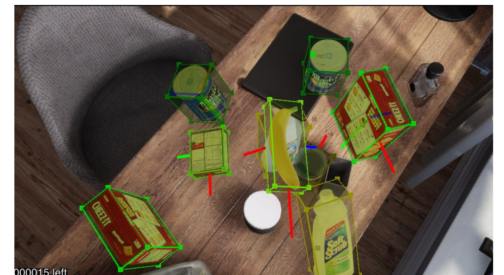
Visualizing the 3D cuboids using NVIDIA Dataset Utilities toolset
