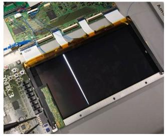
Figure 3. Custom driver applied to AMOLED panel. Bright tapered region across the panel is the 6x540 region driven by the initial circuit prototype.
