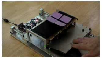
Figure 4. Linear motion platform for tracking and display.
