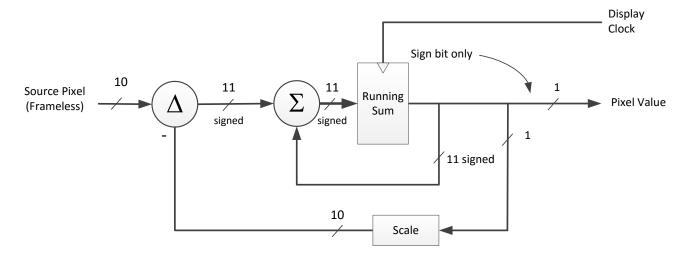
Figure 1. Conventional Delta-Sigma modulation.
