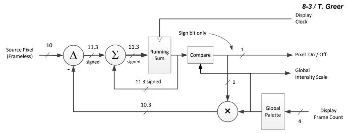
Figure 2. Delta-Sigma with global intensity scaling palette.
